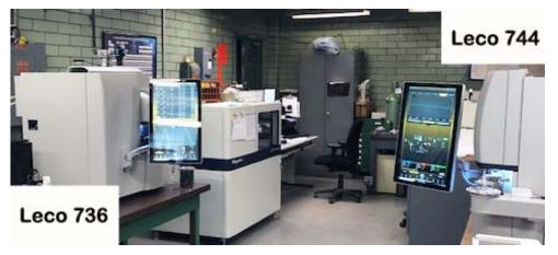
Leco 744 determines carbon and sulfur in metals. Leco 744 takes advantage of the Cornerstone brand software platform an interface to increase usability and lower the cost-per-analysis.
